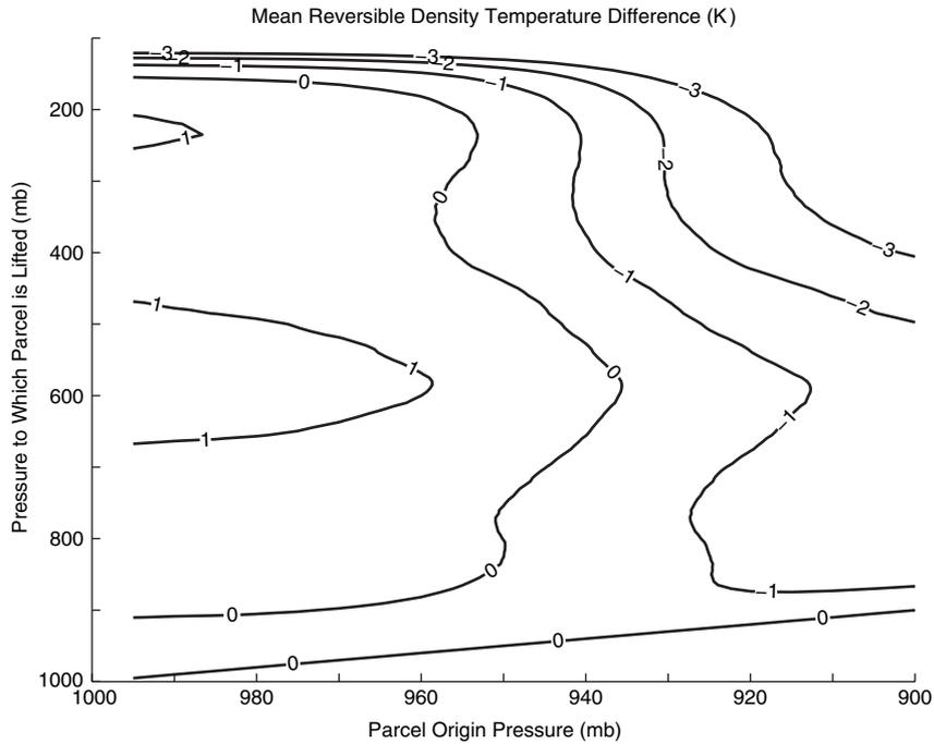
FIGURE 7.1. Contour plot of the difference between the environmental density temperature and the density temperature of a parcel lifted reversibly and adiabatically from the pressure level given on the abscissa to the pressure level on the ordinate. This quantity has been averaged over several thousand soundings taken at Kapingamarangi in the far western tropical Pacific.
