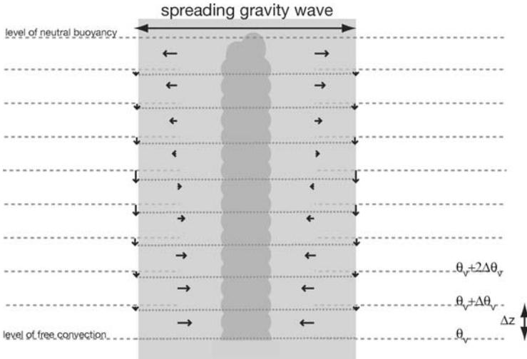
**Figure 10** Schematic of adjustment owing to cumulus heating following Bretherton & Smolarkiewicz (1989). Here the transient adjustment to the moist-adiabatic lapse rate of the convecting tower from Figure 3 is shown to be accomplished by a spreading gravity wave front. As the subsidence wave moves away from the region of convection, it is associated with a downward displacement of isentropes, which equilibrates the buoyancy ( $\theta_v$ ) profile.
