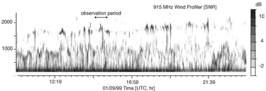
**Figure 7** Signal-to-noise ratio from a 915-MHz wind profiler. At this wavelength, Bragg scattering from humidity gradients dominate the signal, thus illustrating the turbulent structure of the trade-wind boundary layer by highlighting regions of vigorous mixing associated with subcloud thermals and cloud boundaries. Both the trade-inversion and transition layer are evident at this frequency. (Adapted from Kollias et al. 2001.)
