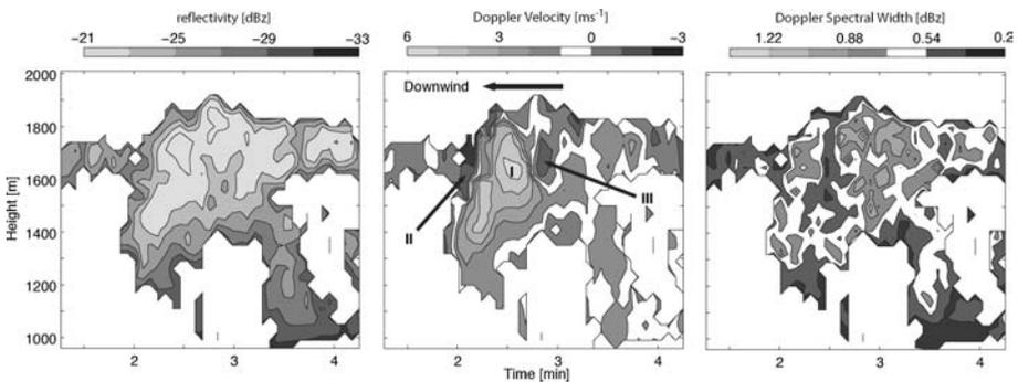
**Figure 8** Radar reflectivities (*left*), Doppler velocities (*center*), and Doppler spectral width (*right*) for a cumulus cloud sampled during the observational period marked in Figure 7. Updrafts and downdrafts are marked on the central panel. Notice the rather broad spectral widths in the updraft core in the rightmost panel. (Adapted from Kollias et al. 2001.)
